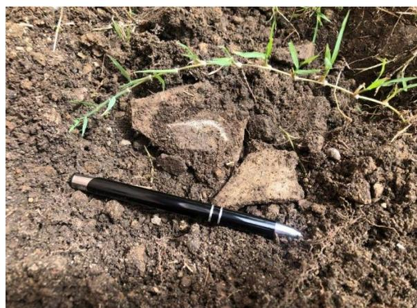
*Fragments of fibro-cement suspected as being ACM buried at shallow depth at the SS2 sampling location outside the administration building's northern face.*
